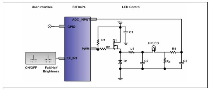
Figure 2-1 Control Circuit
